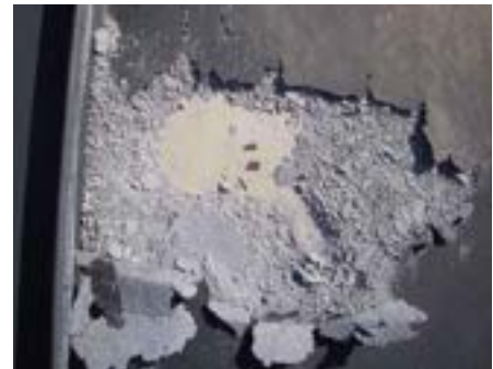
The effect of back side corrosion on zinc.
