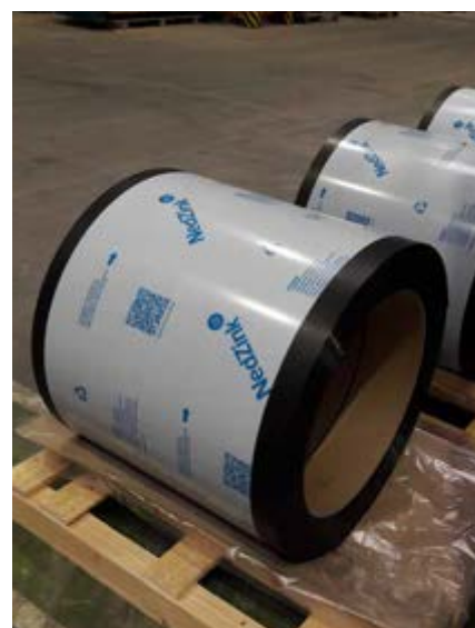
Rolling direction printed on foil
