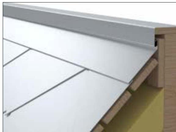
Figure 6.3.13 Details lozenge system on a ventilated substructure.
