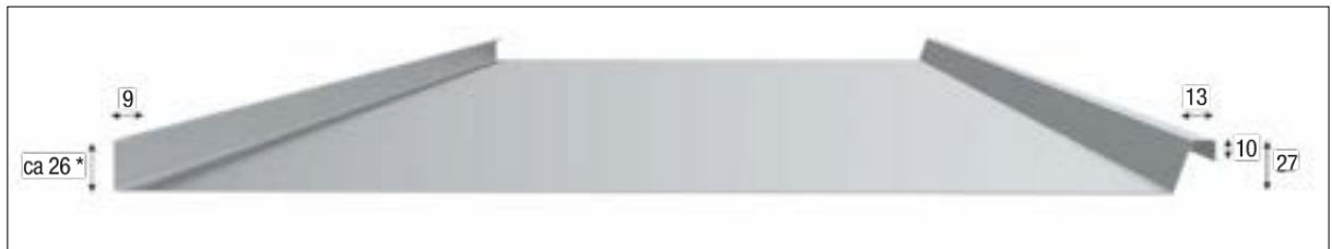
Figure 7.1.2 Standing seam bay
