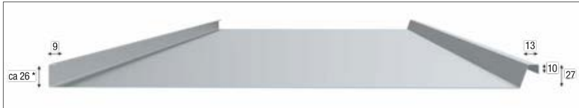
Figure 6.1.2 Dimensions standing seam bay
