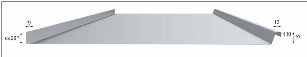
Figure 6.1.2 Dimensions standing seam bay
