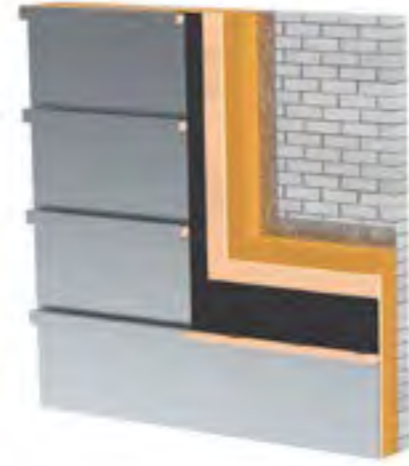
Horizontal roll cap system
