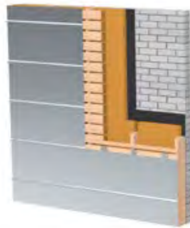
Horizontal standing seam system
