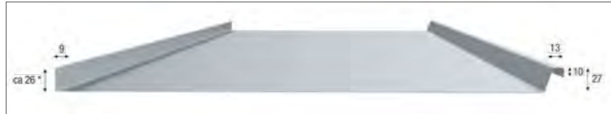
Figure 5.1.2 Dimensions standing seam bay
