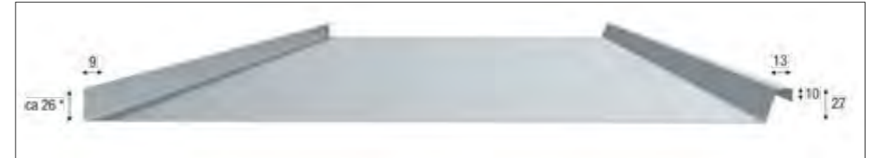
Figure 6.1.2 Dimensions standing seam bay
