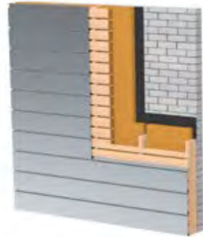
Horizontal Reveal panel system
